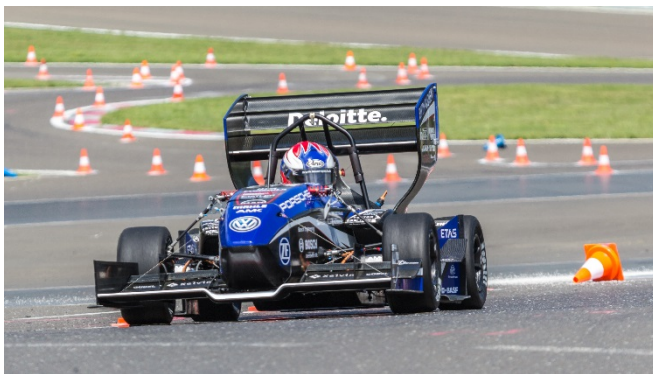
Image 2: No e-mobility without laser technology: Electric racing car "eace05" of the Ecurie Aix - Formula Student Team, RWTH Aachen. It contains laser welded batteries and laser-cut CFK-components. © Ecurie Aix.
