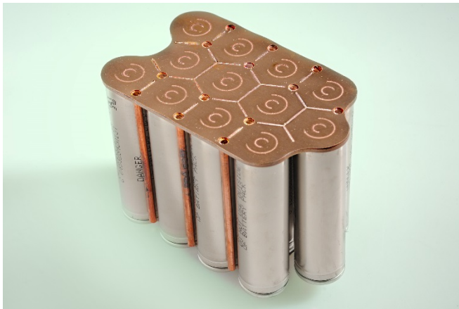
Image 1: LaserTAB: at LASER WoP 2019, Fraunhofer ILT will be demonstrating how to weld battery cells combining a sensitive lightweight robot with laser technology. The laser-welded battery pack was developed in the EU project OPTEMUS (grant number 653288). © Fraunhofer ILT, Aachen, Germany.
